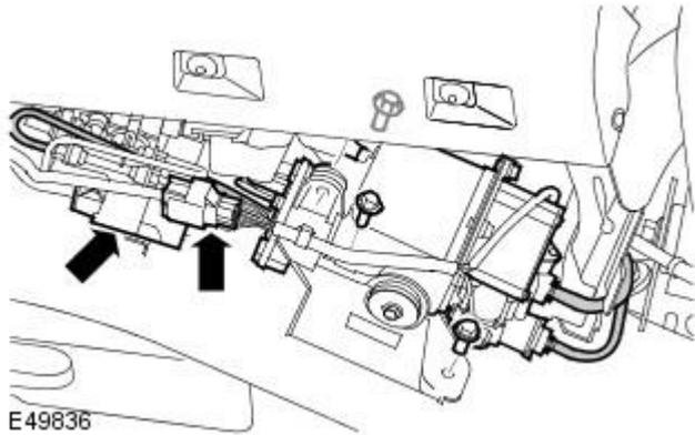
Remove the air suspension compressor.
