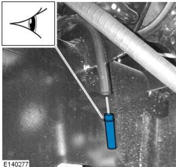
**34.** Install the new air line link pipe.
