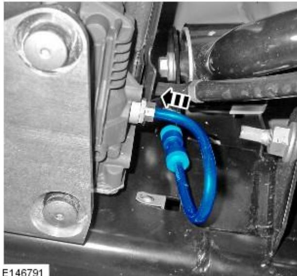
31. Connect the new air line link pipe.
