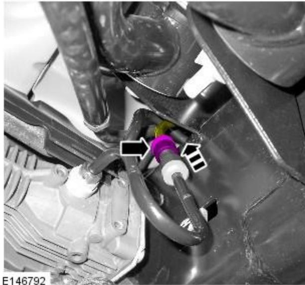
15. Install the new air line link pipe.
