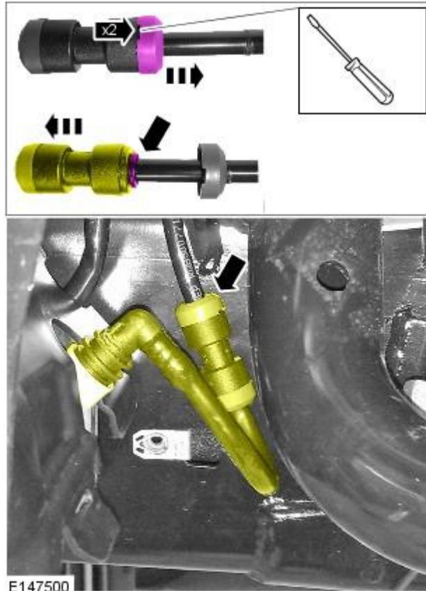
**24.** Disconnect the air line and 2 electrical connectors.
