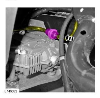
**18.** Connect the air line and 2 electrical connectors.
