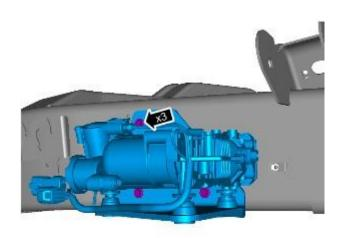
17. NOTE: Suspension compressor upper cover shown removed for clarity.
