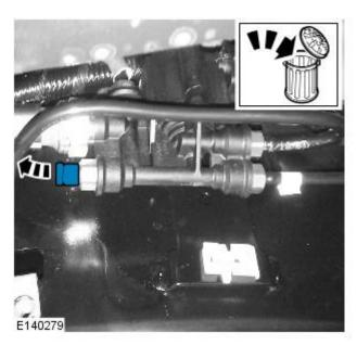
13. CAUTION: Make sure the air line link pipe is correctly fitted. It must be inserted to a depth of 20mm.
