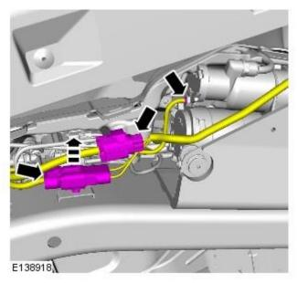
25. CAUTION: Make sure that the 3 suspension compressor mounting nuts in the chassis rail are not damaged or corroded. If required, replace the nuts.
