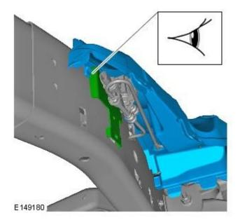
8. CAUTION: Make sure the new pipe is fitted securely into the new air suspension compressor connector, failure to follow this instruction may cause damage to the component.
