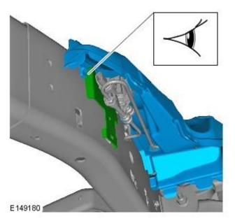
28. CAUTION: Make sure the air lines and wiring are not trapped between the suspension compressor mounting bracket and the chassis, failure to follow this instruction may cause damage to the vehicle.
