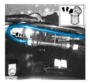
12. CAUTION: Do not remove the blanking plug until after the connector is tightened.
