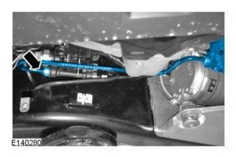
16. CAUTION: Make sure the air lines and wiring are not trapped between the suspension compressor mounting bracket and the chassis, failure to follow this instruction may cause damage to the vehicle.
