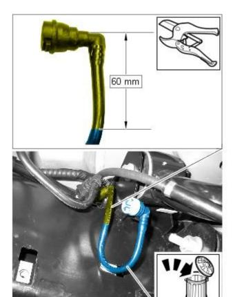
33. CAUTION: Make sure the air line insert is in the correct orientation, failure to follow this instruction may cause damage to the component.
