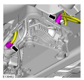
**23.** If installed, remove and discard the air line link pipe.
