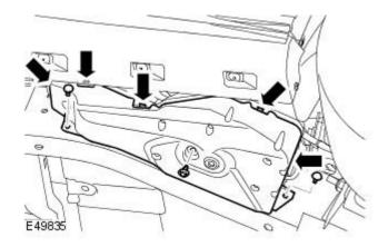
5. CAUTION: Make sure that the 3 suspension compressor mounting nuts in the chassis rail are not damaged or corroded. If required, replace the nuts.
