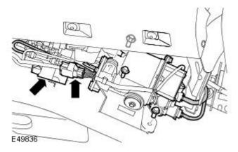
7. CAUTION: Make sure that the cover is correctly located behind the bracket as shown. Failure to follow this instruction may cause noise/vibration issues.
